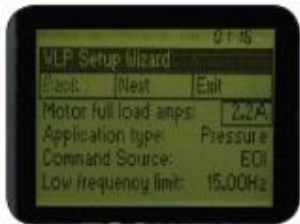
STEP 1: Input Motor's Electrical Specifications
