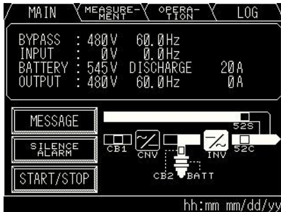
FIGURE 2.7.1 Main screen (Battery operation)
