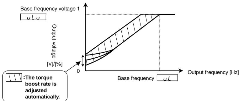
Note: This control system can oscillate and destabilize runs depending on the load. If that should happen, set V/f control mode selection  $P_{\tau}$  to 0 (Constant torque characteristics) and increase torque manually.
