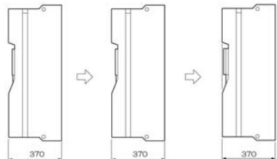
Note: The inverters of these capacities come equipped with an Add-on type option case as standard. When installing an optional Add-on type device, remove the case.
