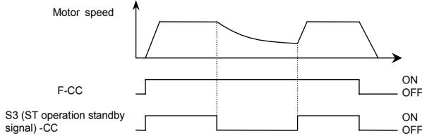
$U_{U5}=2$ : This function operates after the S3-CC terminal connection has been opened first and then connected again.
