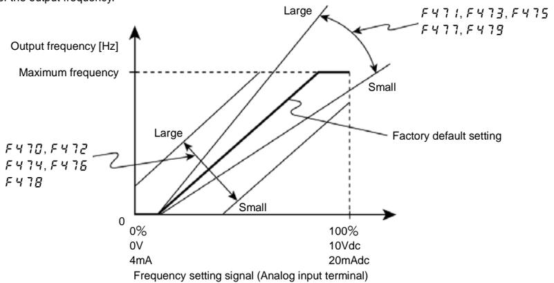
Bias adjustment of analog input terminals (*F470, F472, F474, F476, F478*)
