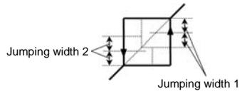
During acceleration or deceleration, the jumping function is disabled for the operation frequency.
