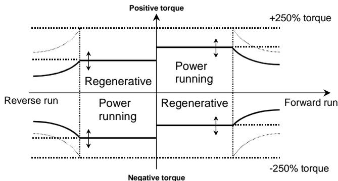
The torque limits can be changed arbitrarily by means of external signals.
