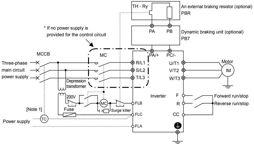
Note 1: Connection when using an MCCB with a top coil instead of an MC.
