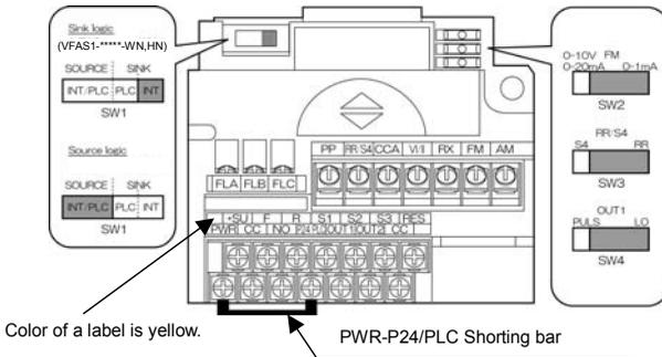
⇒ How to set input terminal function, refer to section 7.
