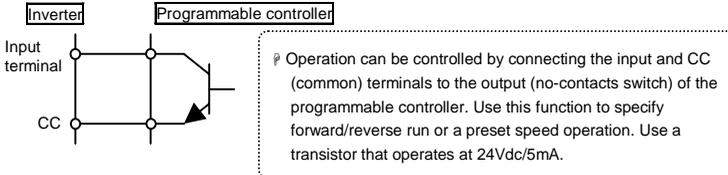
\* Interface between programmable controller and inverter
