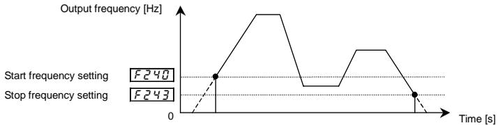
Note: Set these parameters so that the start frequency **F240** is higher than the stop frequency **F243**.
