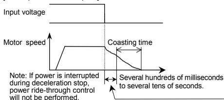
The time for which the operation of the motor can be continued depends on the machine inertia and load conditions. Before using this function, therefore, perform verification tests. Use with the retry function allows the motor to be restarted automatically without being brought to an abnormal stop.
