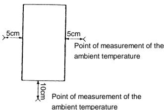
Note: The inverter is a heat-emitting body. Make sure to provide proper space and ventilation when installing in cabinet. When installing inside a cabinet, we recommend the removal of the protective cover.
