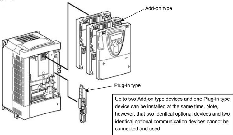
Depending on the capacity, the installation of an Add-on type device may increase the depth of the inverter.
