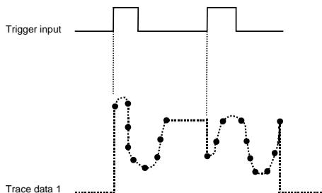
Ex.) When using the RR/S4 terminal as the tracing back trigger signal terminal
