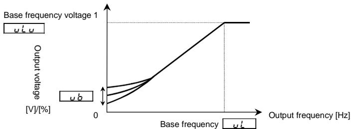
\* To increase the torque further, increase the setting value of the manual torque boost parameter u<sub>b</sub>.
