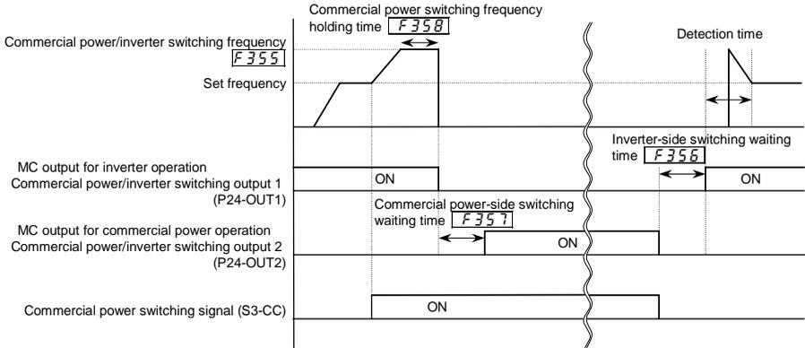
Commercial power switching signal S3-CC ON : Commercial power operation
