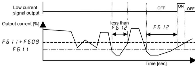
When **F610=1** (tripping), the inverter will trip if low current lasts for the period of time set with **F612**.
