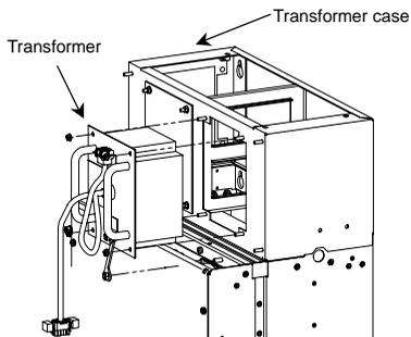
Mount the transformer case on an inner wall of the cabinet and secure the transformer to the case with screws.
