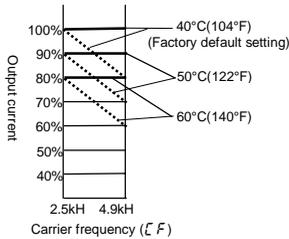
• Standard installation without top cover or side-by-side installation without top cover
