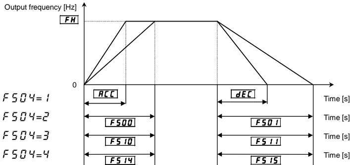
Acceleration/deceleration time 1 is initially set as the default. Acceleration/deceleration time 2, 3 and 4 can be selected by changing the setting of the F504.
