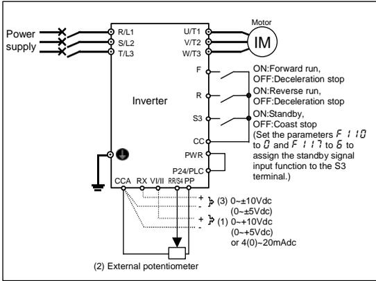
⚠ The inverter is factory-configured so that, if F and R are turned on at the same time, the inverter will stop operation. If necessary, the direction of rotation can be reversed by changing parameter settings. ⇒ Refer to Section 6.2.1.
