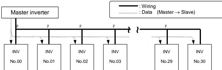
: Use the terminal board to branch the cable.
