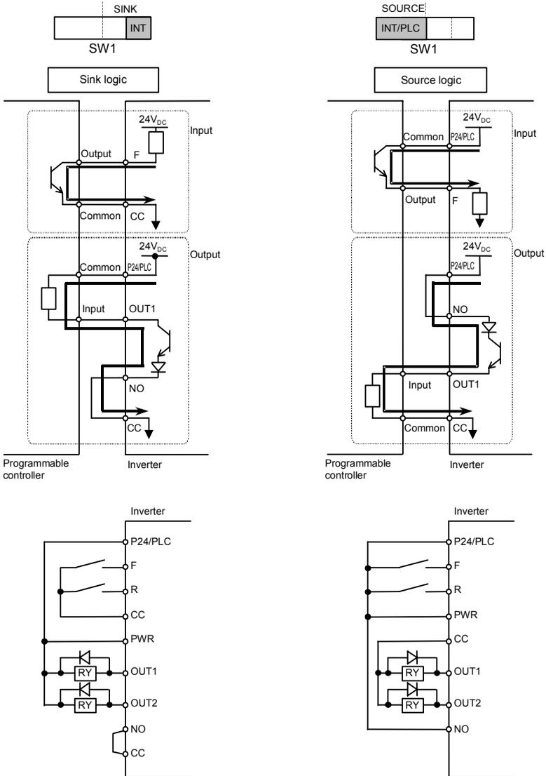
**■ Sink logic/source logic (When an external power supply is used)**
