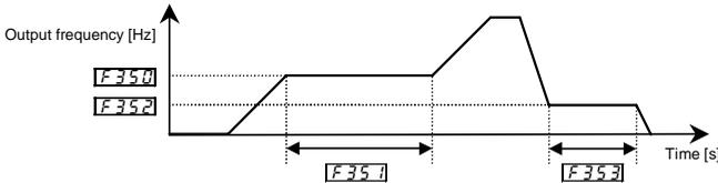
2) To suspend acceleration or deceleration by means of a signal from an external control device
