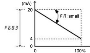
The analog output inclination can be adjusted using the parameter  $FN$ .
