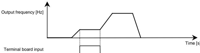
Ex.) When using the RR/S4 terminal as the acceleration/deceleration suspend terminal
