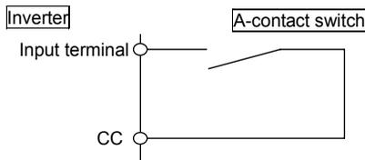
This function is activated when the input terminal and CC (common) are short-circuited. Use this function to specify forward/reverse run or a preset speed operation.
