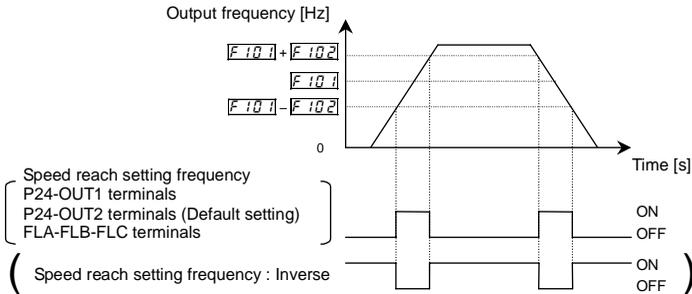
2) If the detection band value + the set frequency is more than the designated frequency
