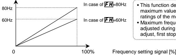
• This function determines the maximum value in line with the ratings of the motor and load.
