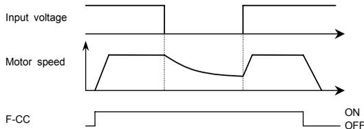
$U 5 = 1$ : This function operates after power has been restored following detection of an undervoltage by the main circuits and control power.
