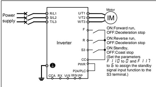
ⓘ The inverter is factory-configured so that, if F and R are turned on at the same time, the inverter will stop operation. If necessary, the direction of rotation can be reversed by changing parameter settings. ⇒ Refer to Section 6.2.1.
