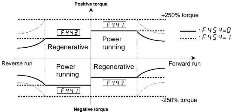
With the parameter *F454*, you can select the item that is limited in the constant output zone (somewhat weak magnetic field) from between constant output (*F454=0*: default setting) and constant torque (*F454=1*). When you select the constant torque limit option, you should preferably select the output voltage limit option (*F307=3*) with the parameter *F307* (base frequency voltage selection).
