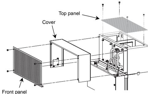
Secure the cover, front panel and top panel to the transformer case with screws.
