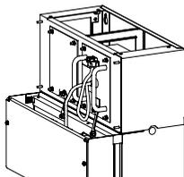
Connect the transformer connector on the drive. Then connect the supplied earth wire.
