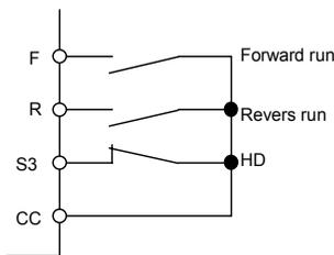
Forward run (F): If you press the Forward (F) button, the motor rotates in the forward direction at the frequency specified with a command.
