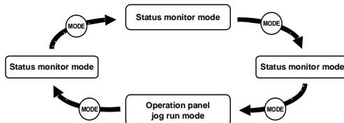
Note1: When the inverter is in operation (RUN key lamp is lit) or when an operation command is issued (RUN key lamp is lit), the inverter cannot be switched to operation panel jog run mode.
