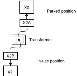
VFAS1-6400KPC to 6630KPC drives feature 2 transformers. Make this connection for each transformer.
