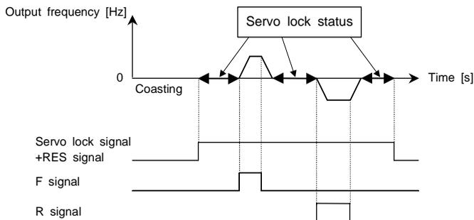
Even if the motor is started with servo lock activated, a starting torque of 150% or more can be produced.
