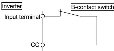
This function is activated when the input terminal and CC (common) are open-circuit. Use this function to specify operation standby signal or reset signal.
