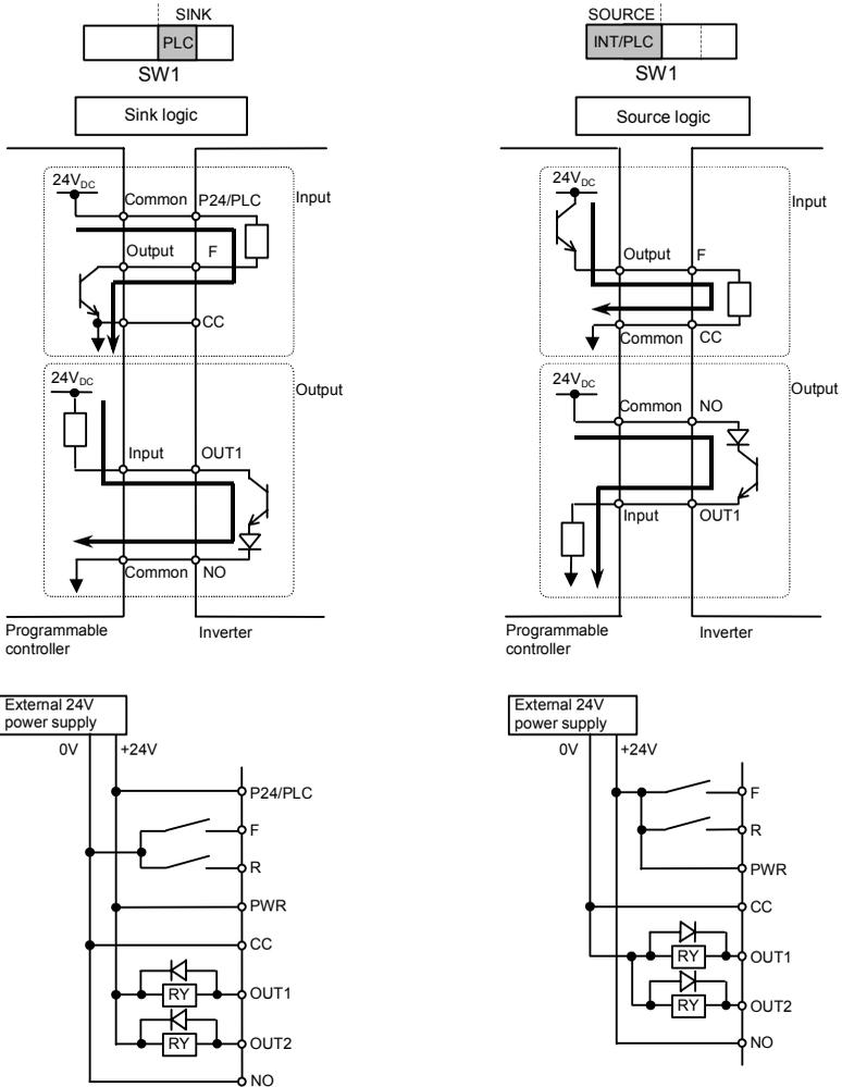
**Note: Be sure to connect the 0V terminal on the external power supply to the CC terminal on the inverter.**
