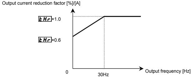
Note: The motor overload starting level is fixed at 30Hz. If necessary, set  $\boxed{\text{OLn}}$  to 4, 5, 6 or 7. (See the following section.) Even if the inverter is used with a Toshiba standard motor, the load may need to be reduced at frequencies of 30Hz and below in some cases. In such cases, set  $\boxed{\text{OLn}}$  to 4, 5, 6 or 7 and set the  $\boxed{\text{OL}}$  reduction starting frequency ( $\boxed{\text{F505}}$ ) according to the motor.
