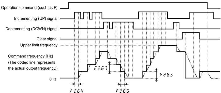
■ **If two signals are input simultaneously**
