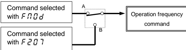
A : Selects the command set with parameter *F 00d*. – Operation frequency command switching terminal OFF
