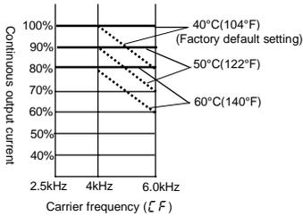
• Standard installation without top cover or side-by-side installation without top cover.
