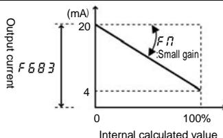
The analog output inclination can be adjusted using the parameter **F683**
