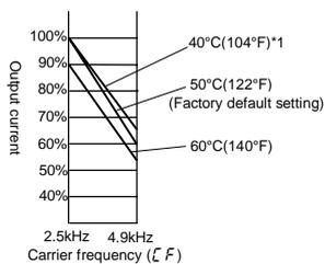
\*1: It is current reductions curve, when setting a parameter F531 as 1.
