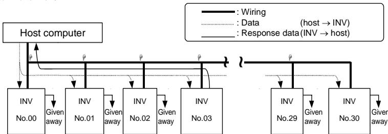
"Given away": Only the inverter with the selected inverter number conducts data processing. All other inverters, even if they have received the data, give it away and stand by to receive the next data.
