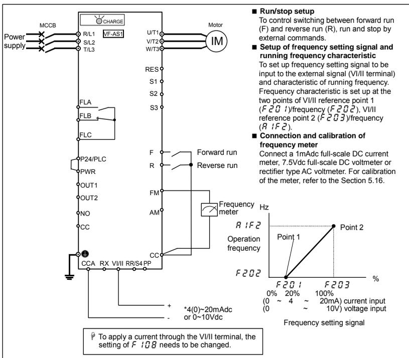
**7.3.3 Setup by analog input signals (RX terminal)**
