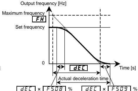
Both the S-pattern lower-limit setting (F 5 0 6, F 5 0 8) and the S-pattern upper limit setting (F 5 0 7, F 5 0 9) affect all acceleration/deceleration pattern settings.
