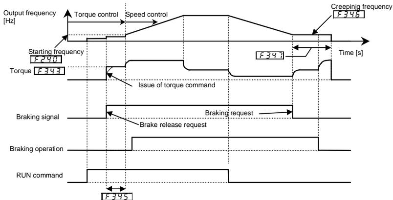
Ex.) When using the OUT1 terminal as the brake signal output terminal
