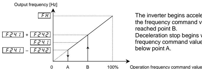
The inverter begins accelerating after the frequency command value has reached point B. Deceleration stop begins when the frequency command value decreases below point A.
