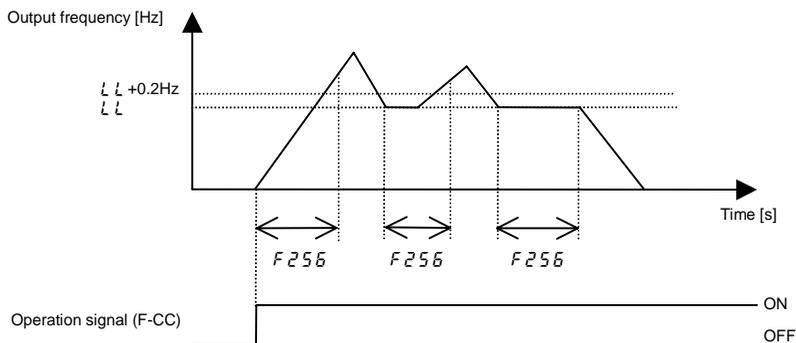
Note: This function is enabled even at the start of operation and during switching between forward and reverse run.
