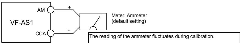
It is recommendable to use an ammeter with a current rating 1.5 or more times as high as the output current rating of the inverter.
