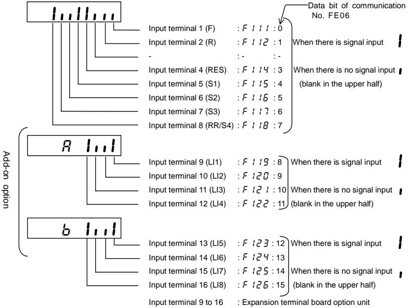
Note: When F 1 0 7 is set at a number of 1 to 8 expansion terminal board option input terminal information (A, b) indicate information of lower 8 bit terminal (B0-B7).
