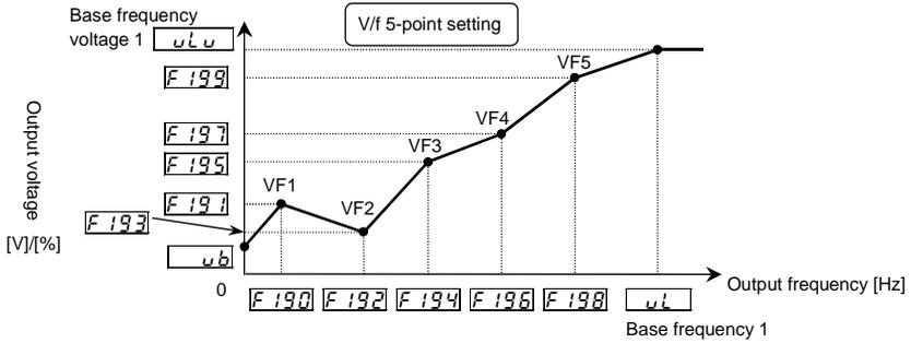
Note 1: Restrict the amount of torque to boost ( $\omega b$ ) to 3% or so. Boosting the torque too much may impair the linearity between points.
